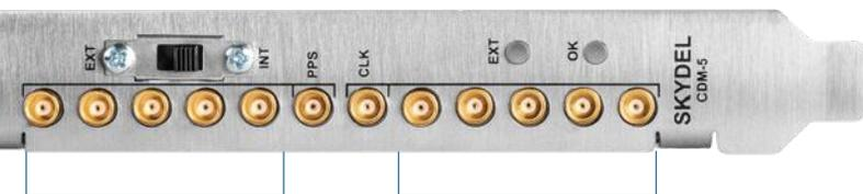
CDM-5 can synchronize up to 5 devices using 10MHz and 1PPS signals
